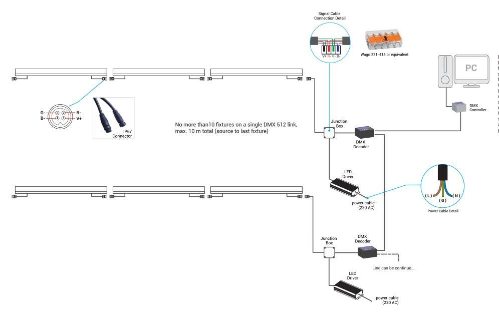
Data cabling from DMX source to first fixture and between subsequent BAYLINE fixtures shall be Cat5e UTP or higher (stranded type only) or other cable type suitable for DMX communication. Consult DMX standard for additional guidance.
